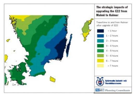
Isocrones for travel to and from Kalmar after the E22 has been upgraded to motorway standard between Malmö and Kalmar.
