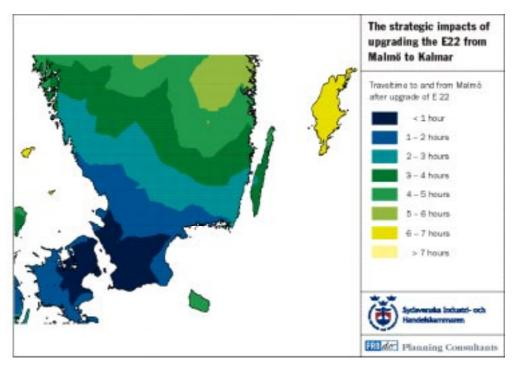
Isocrones for travel to and from Malmö after the E22 has been upgraded to motorway standard between Malmö and Kalmar.
