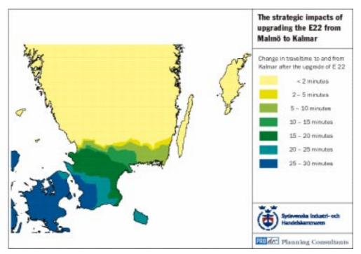
The decrease in travel time to and from Kalmar as a consequence of the upgrade of E22 to motorway standard between Malmö and Kalmar.
