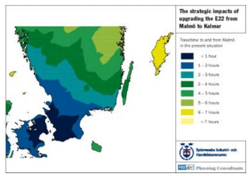
The general structure of the Swedish road network can easily be seen on the isocrone map where the E6 are stretching the isocrones towards Göteborg, the E4 are stretching the isocrones towards Jönköping (and Stocholm) and the E22 are stretching the isocrones towards Kristianstad and Kalmar.
